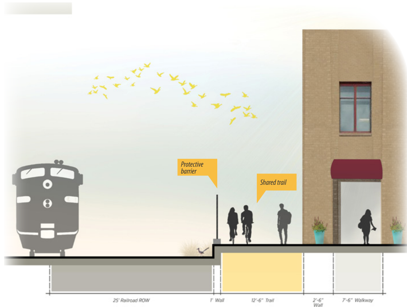
FIGURE 10. Typical Section East Along Railroad Tracks
